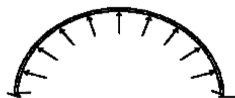
Figure 13 Curved plate with water pressure at the inner wall. Plate acts like a membrane
