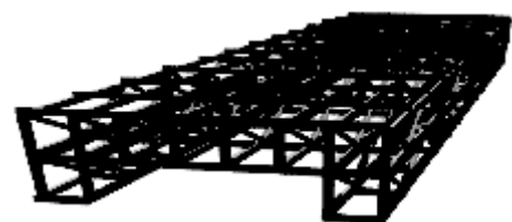
Figure 12 Truss structure of FRP hull
